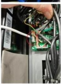
For the SG-ready heatpumps and P13 and P17 horizontal you can use a two core wire (max 0,75mm<sup>2</sup>). For the heatpumps with a small pcb you need cable 7021825 to connect directly on the PCB. Only the black and blue are used(It is ok to cut off the green and brow, but be sure they don't touch each other).
