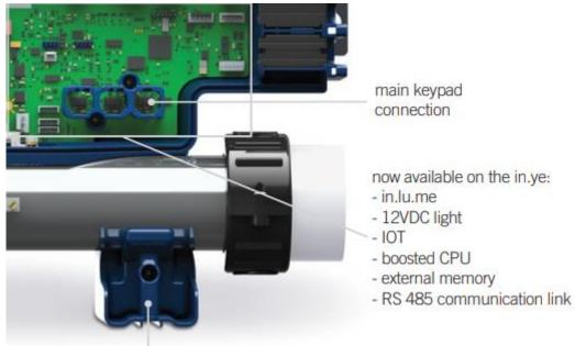
The control box stay in place. The In.Grid's cable needs to plug in to one of the free CO-port.
