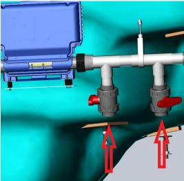
• after connecting the pipe (leave 10 min for the glu to can dry), get down the hollanders and fill the system with water (deair it)
